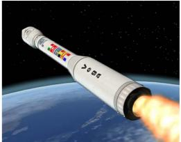
Vega's second and third stages are based on Zefiro solid-propellant motors developed by Avio, respectively called P80FW (first stage), Zefiro-Z23 (2<sup>nd</sup>) and Zefiro-Z9A (3<sup>rd</sup>).
