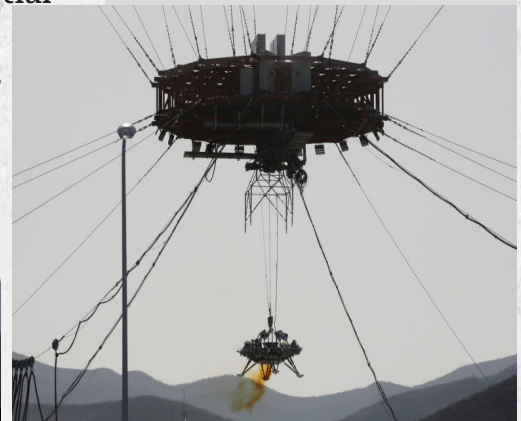
Hover drop test under the rig.
